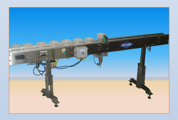
This style conveyor moves containers with an intermittent motion. This is ideal for conveying tapered cups. An optional rising table at the fill zone allows the cups to be lifted to the filler's nozzle to bottom up fill viscous products. The conveyor is all pneumatic and can be made in various lengths. Shown above is 10 ft. long x 6" wide. Cup densters and plastic film sealers can be added.
