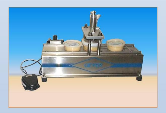
The CP-2 indexes the cups under the presser head and presses hand paced lids securely onto the cup and then moves it. Operates by compressed air.
